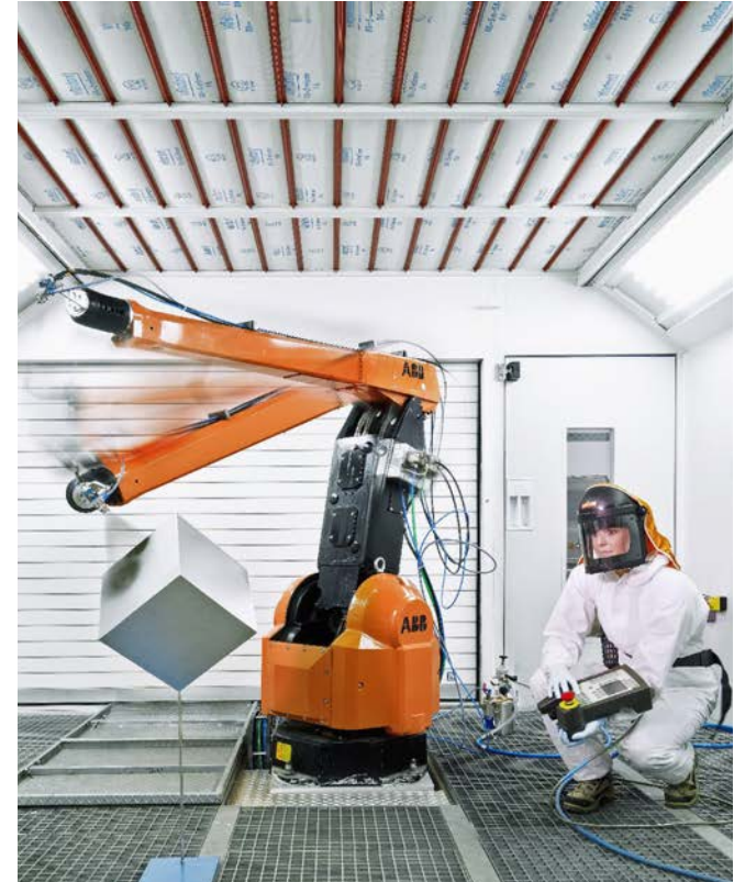
Spray robot at INM for the application of nano-coatings
